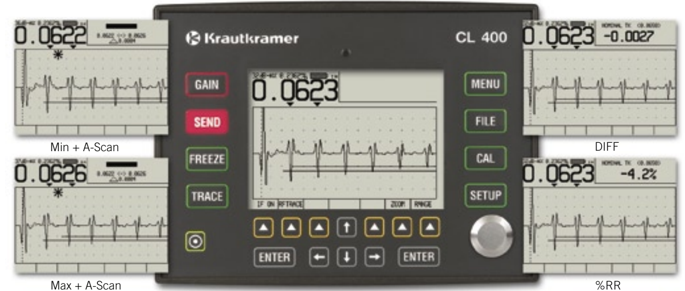
A-Scan option provides a variety of views beyond the above THICKNESS + A-SCAN View
