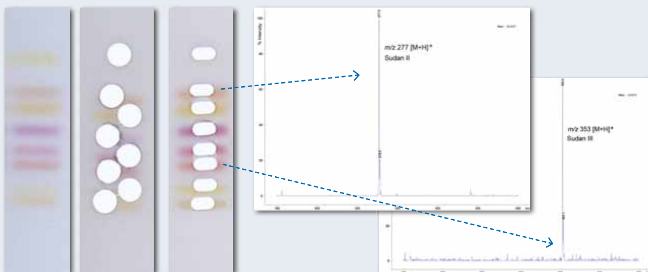
The oval elution head is preferable for narrow, closely neighboured zones.
