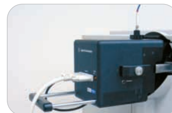
Pulsed Dynamic Focusing MALDI (PDF-MALDI) Source
