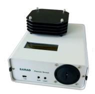
The required fast exchange rate of sampled air is realized by a highly permeable chamber placed outside the instruments enclosure. The relative Thoron sensitivity is comparable with the one of pump based instruments.
