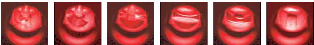
Sequences of the integrated color camera in the graphite furnace
