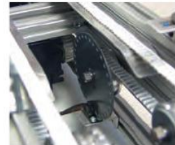
Encoding Disk with optic Sensor
